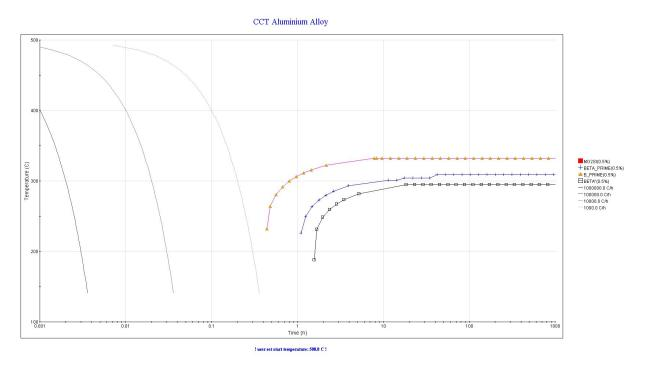
Calculated CCT diagram for the 356 alumnium alloy.
